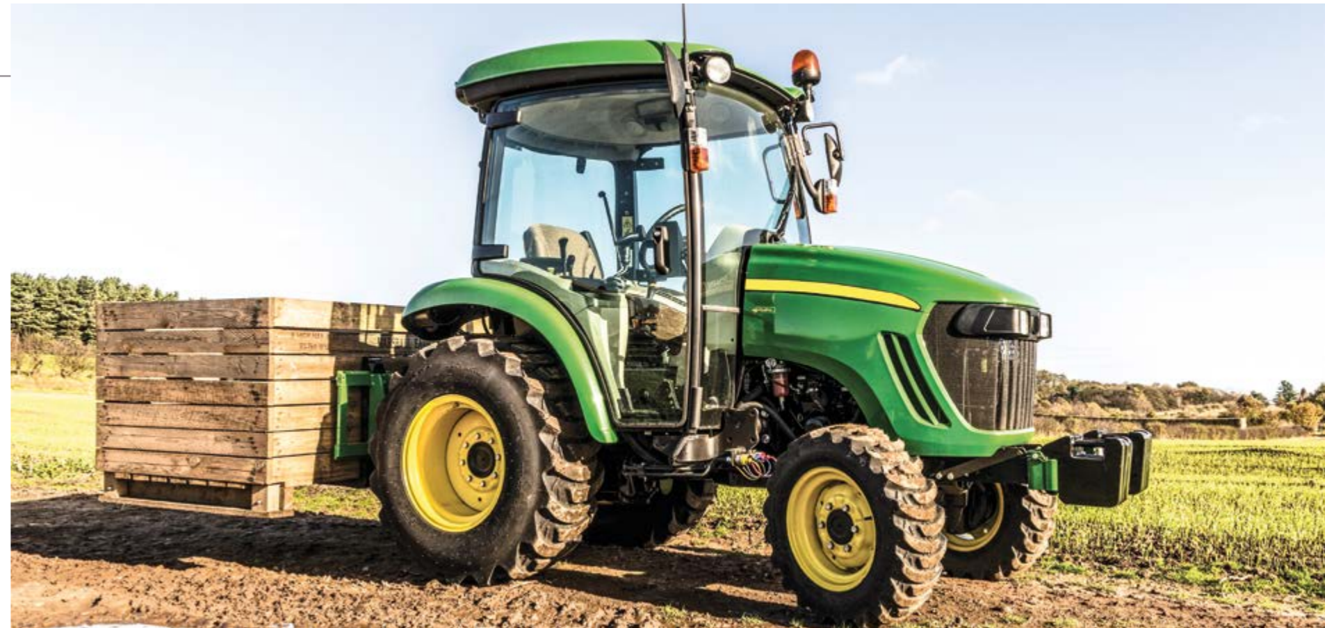
*Tractor fitted with HME rear linkage mounted pallet forks and compact front weights.
